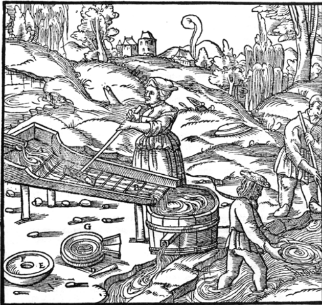
A—HEAD OF THE SLUICE. B—RIFFLES. C—WOODEN SCRUBBER. D—POINTED STICK. E—DISH. F—ITS CUP-LIKE DEPRESSION. G—GROOVED DISH.
