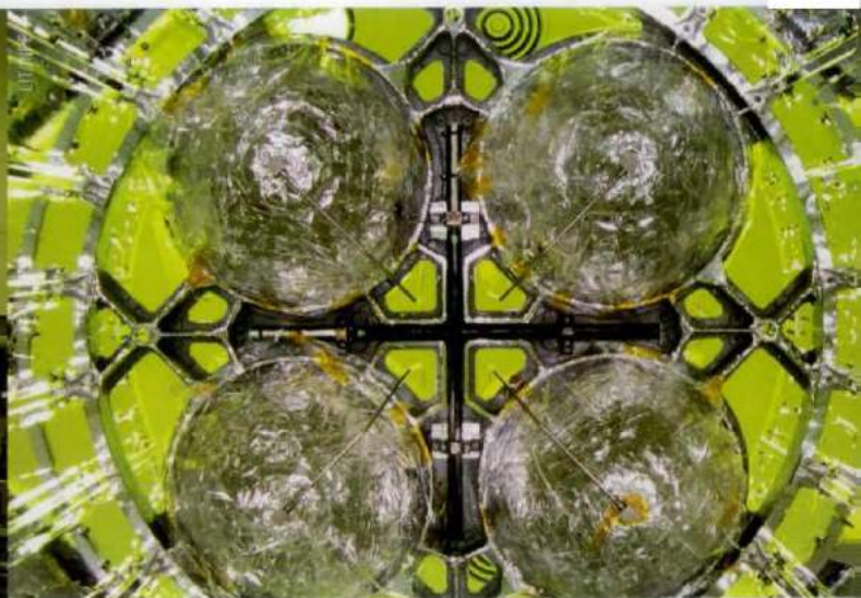
Hydrazine fuel tanks mounted on the central cylinder.
