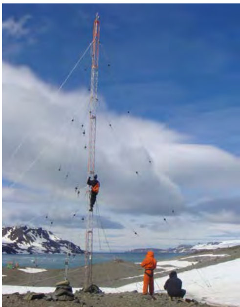
Ionosonde installed at the Keller Peninsula, King George Island, near to the Comandante Ferraz Antarctic Station. Photo: Emília Correia (INPE/UPM).
